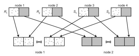
Fig. 14.15 Example of Parallel Hash Join
