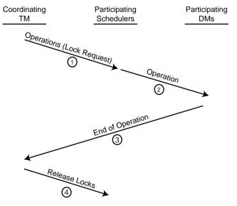
Fig. 11.10 Communication Structure of Distributed 2PL
