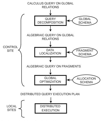
Fig. 6.3 Generic Layering Scheme for Distributed Query Processing
