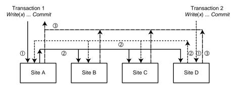
**Fig. 13.3** Eager Distributed Replication Protocol Actions. (1) Two *Write* operations are applied on two local replicas of the same data item; (2) The *Write* operations are independently propagated to the other replicas; (3) Updates become permanent at commit time (shown only for Transaction 1).
