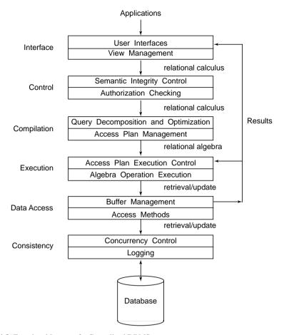
Fig. 1.9 Functional Layers of a Centralized DBMS
