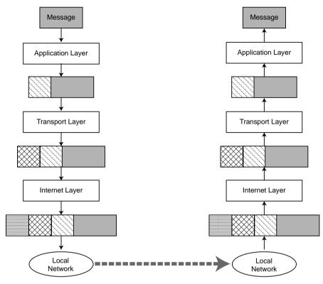
Fig. 2.18 Message Transmission using TCP/IP
