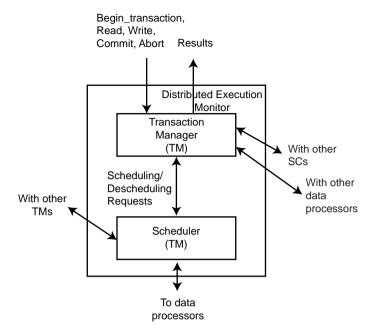
Fig. 10.5 Detailed Model of the Distributed Execution Monitor
