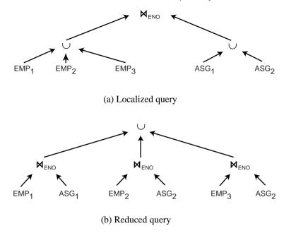
Fig. 7.7 Reduction by Horizontal Fragmentation (with Join)
