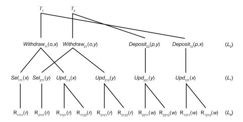
Fig. 11.19 Multilevel Transaction Example (Based on [Weikum, 1991])
