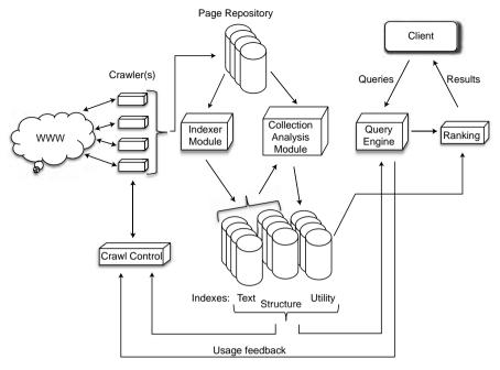
Fig. 17.4 Search Engine Architecture (Based on [?]
