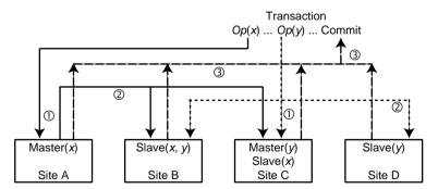
**Fig. 13.2** Eager Primary Copy Replication Protocol Actions. (1) Operations (*Read* or *Write*) for each data item are routed to that data item's master and a *Write* is first applied at the master; (2) *Write* is then propagated to the other replicas; (3) Updates become permanent at commit time.
