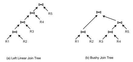
Fig. 9.3 Left Linear versus Bushy Join Tree
