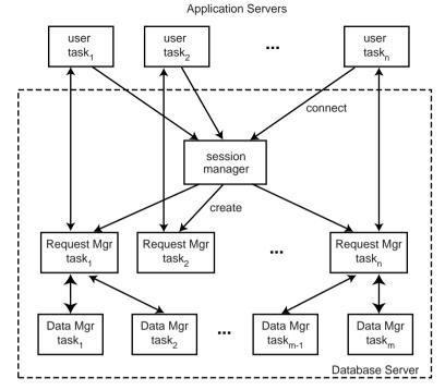
Fig. 14.2 General Architecture of a Parallel Database System
