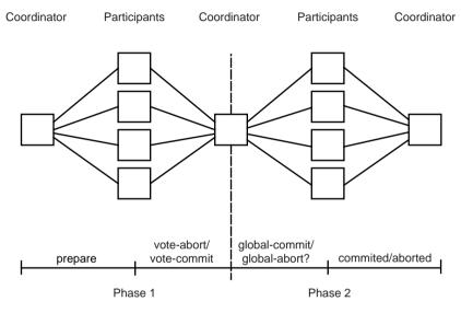
Fig. 12.11 Centralized 2PC Communication Structure
