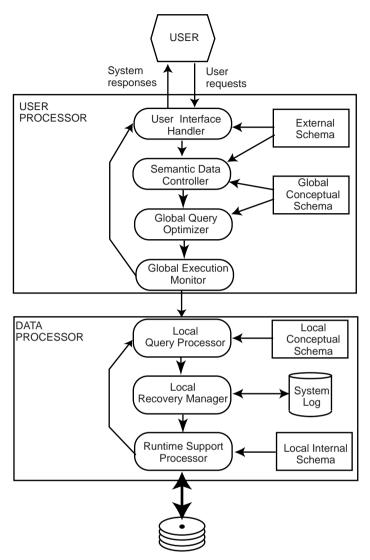
Fig. 1.15 Components of a Distributed DBMS
