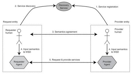
**Fig. 17.12** A typical Web Service workflow suggested by the W3C Web Services Architecture (Based on [Booth et al., 2004].)
