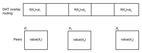
Fig. 16.5 DHT-based P2P Network
