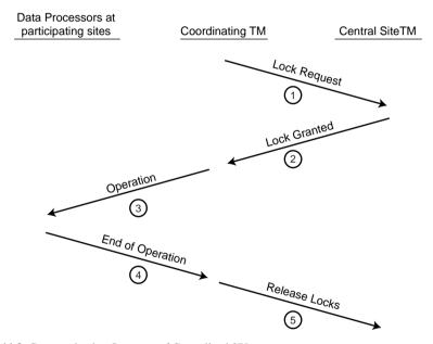
Fig. 11.9 Communication Structure of Centralized 2PL
