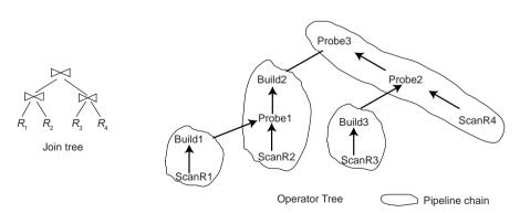
Fig. 14.19 A join tree and associated operator tree
