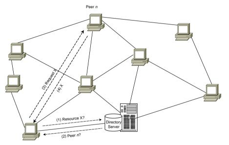
**Fig. 16.3** Search over a Centralized Index. (1) A peer asks the central index manager for resource, (2) The response identifies the peer with the resource, (3) The peer is asked for the resource, (4) It is transferred.
