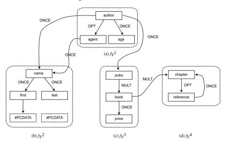
Fig. 17.20 Example Vertical Fragmentation of Schema
