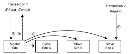
**Fig. 13.4** Lazy Single Master Replication Protocol Actions. (1) Update is applied on the local replica; (2) Transaction commit makes the updates permanent at the master; (3) Update is propagated to the other replicas in refresh transactions; (4) Transaction 2 reads from local copy.
