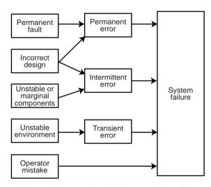
Fig. 12.2 Sources of System Failure (Based on [Siewiorek and Swarz, 1982])
