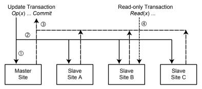
**Fig. 13.1** Eager Single Master Replication Protocol Actions. (1) A *Write* is applied on the master copy; (2) *Write* is then propagated to the other replicas; (3) Updates become permanent at commit time; (4) Read-only transaction's *Read* goes to any slave copy.
