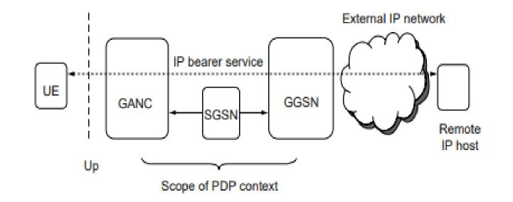
Figure 3.4 End-to-end QoS architecture.
