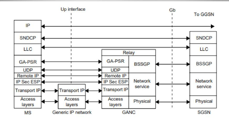
Figure 3.3 Up PS Domain User Plane Protocol Architecture. (From Generic Access to the A/Gb Interface; Stage 2 (Release 7), 3GPP TS 43.318, November 2006.)
