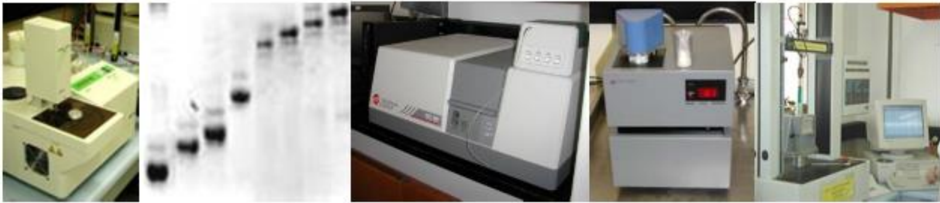
Figure 3. Cooking quality assessment. From left to right: calorimeter, molecular marker products indicating different grain qualities, UV-vis spectrometer, viscometer and texture analyser.
