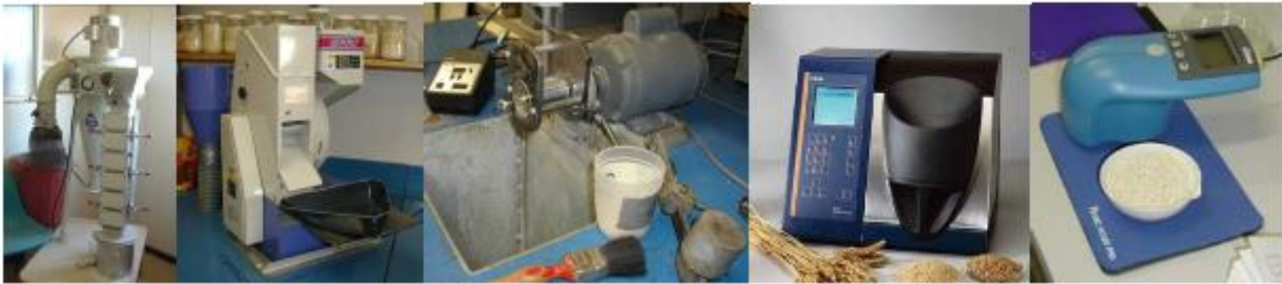
Figure 1. Physical quality assessment. From left to right: aspirator, dehusser, mill, image analysis and the spectrophotometer.
