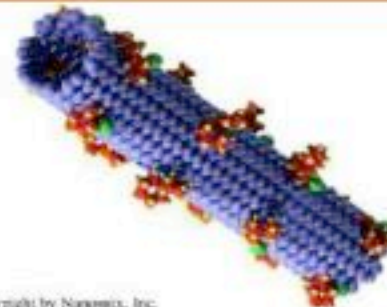
Figure 13. A functionalized single wall carbon nanotube as an H_2 gas sensor by Nanomix ( www.nano.com ).
