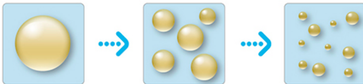
Top-down (rupturing large droplets)
