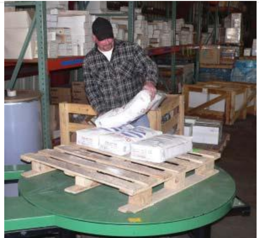
A fixed-height turntable for pallets with short low stacks
