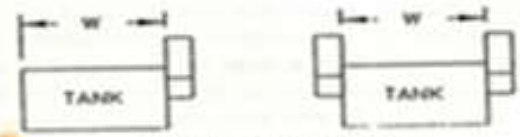
SLOT ON TANK Q = CLW ONE-HALF Q IN EACH SLOT IF SLOTS ON BOTH SIDES
