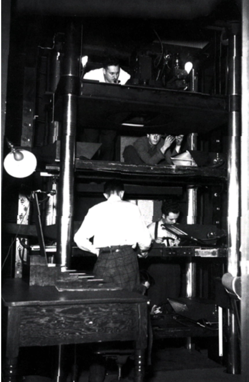
The multiplane camera added an illusion of three-dimensionality to Disney films, beginning with "The Old Mill" (1937).
