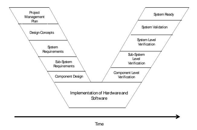
While this model may not precisely match the design process for any single designer, it does represent the generic steps that should be followed when dealing with the design of an integrated system. The advantage of understanding the design process in a generic manner is that key milestone dates can be identified. Once the key milestone dates are determined, it is then possible to identify the timing of Concurrent Engineering activities to ensure reliability requirements are being addressed.
